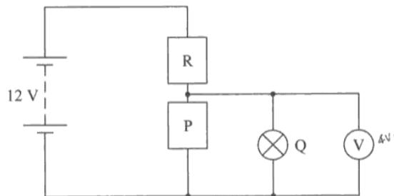
The supply has a negligible internal resistance. The reading on the voltmeter is 4.0 V.
