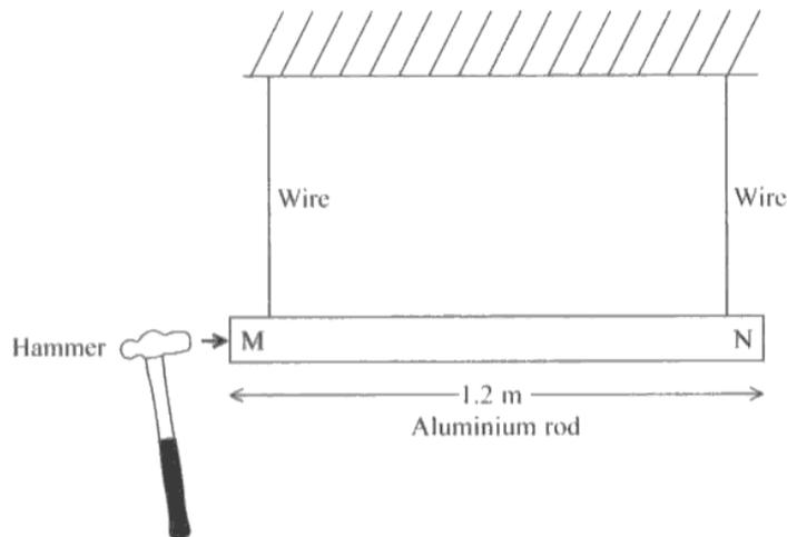
A wave pulse is made to travel along the rod and reflect from end N. The wave pulse is produced by hitting end M gently with a hammer so that the hammer remains in contact with end M until the reflected pulse returns.
